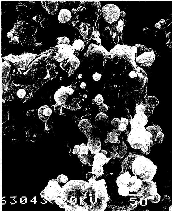
Fig. 6. SEM of freshly spray-dried micropellets dealing with formulation 17.
