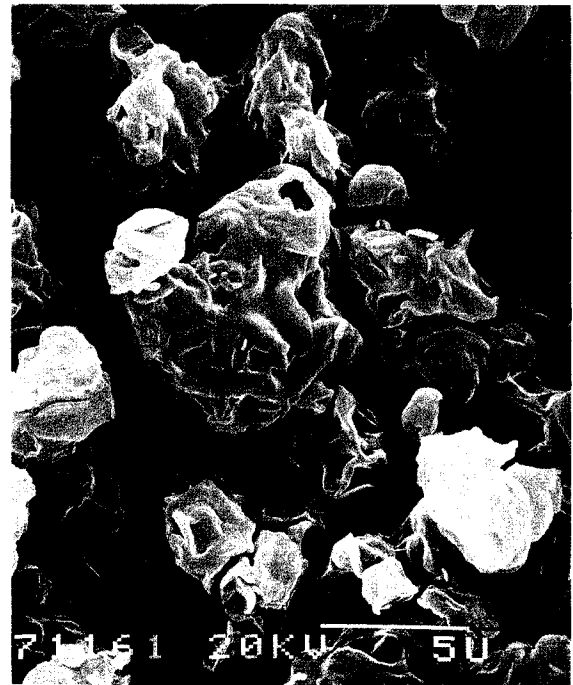
Fig. 9. SEM of freshly spray-dried micropellets dealing with formulation 21.
