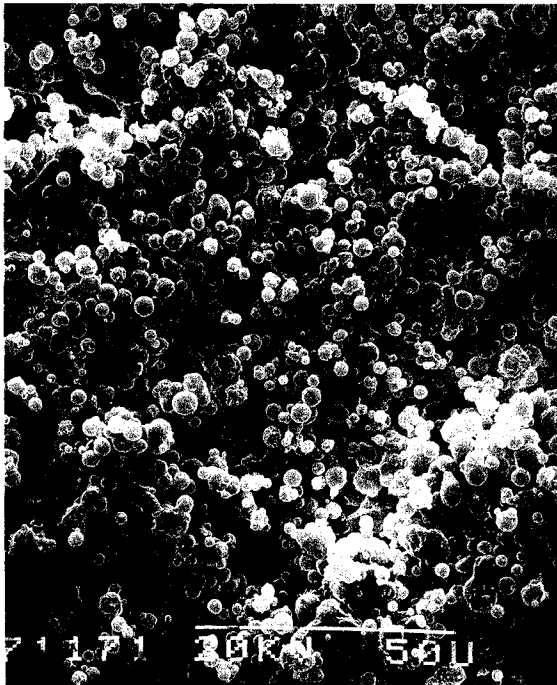
Fig. 7. SEM of freshly spray-dried micropellets dealing with formulation 18.
