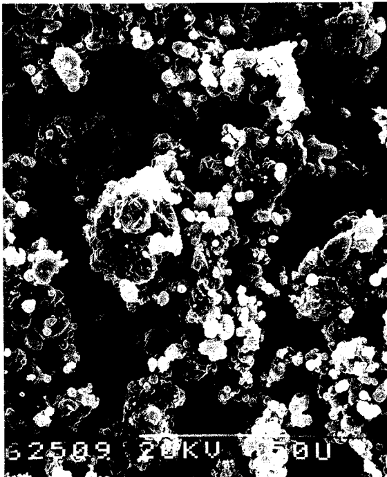
Fig. 3. SEM of freshly spray-dried micropellets dealing with formulation 12.
